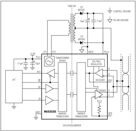
Figure 5. A typical application circuit for the MAX3535E.
