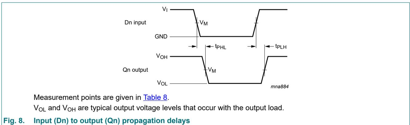
Octal D-type transparent latch with 5 V tolerant inputs/outputs; 3-state
