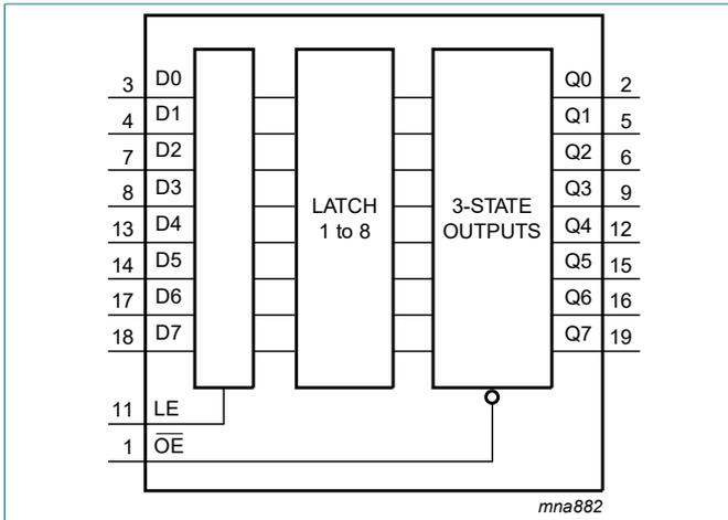
Fig. 3. Functional diagram
