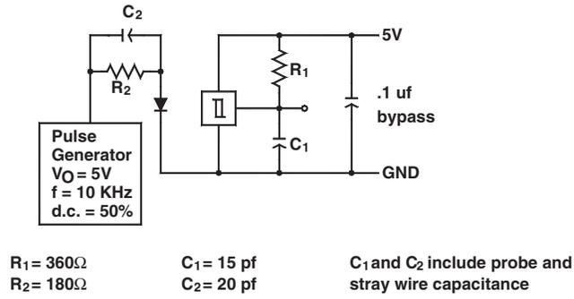
Fig. 9 Switching Times Definition for Buffers
