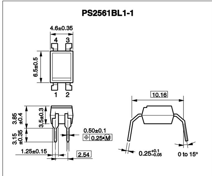
Lead Bending Type (Gull-Wing)
