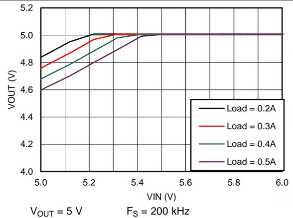
Figure 68. Dropout Curve
