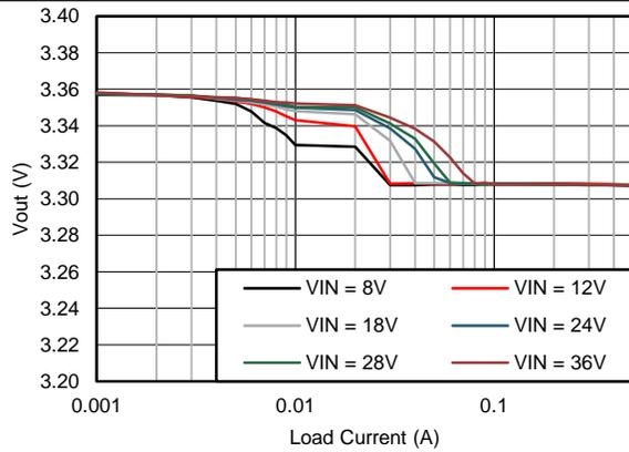
Figure 7.  $V_{OUT}$  Regulation
