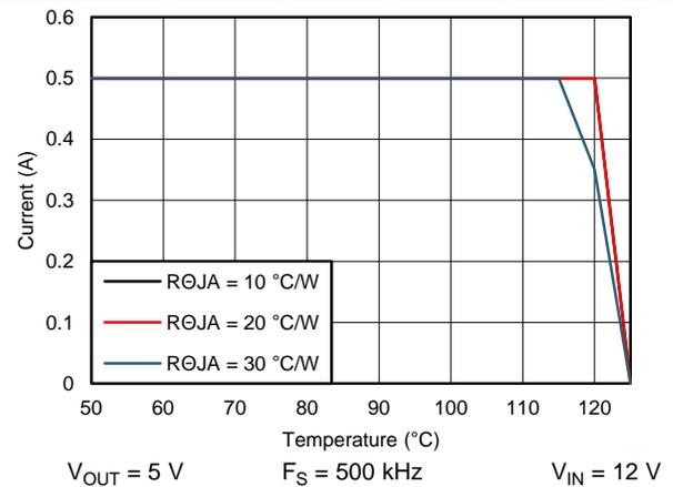
Figure 64. Derating Curve
