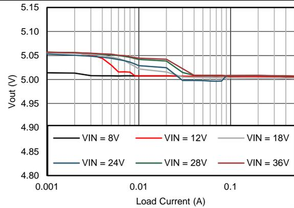
Figure 8.  $V_{OUT}$  Regulation
