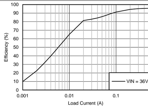
$V_{OUT} = 24\text{ V}$   $F_{SW} = 500\text{ kHz}$
