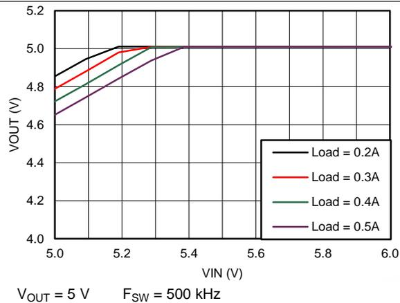
Figure 15. Dropout Curve
