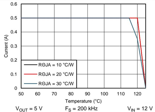
Figure 70. Derating Curve
