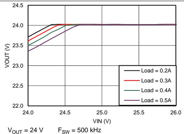
Figure 18. Dropout Curve
