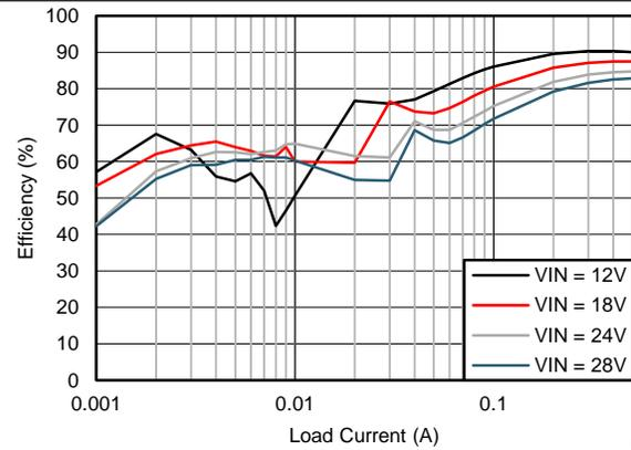
$V_{OUT} = 5\text{ V}$   $F_{SW} = 1\text{ MHz}$
