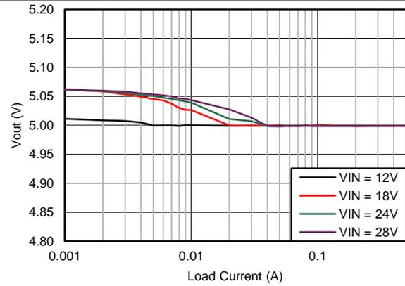
Figure 10.  $V_{OUT}$  Regulation
