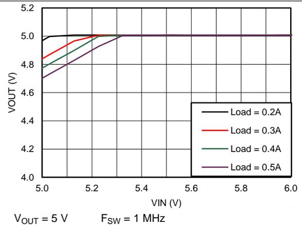
Figure 16. Dropout Curve
