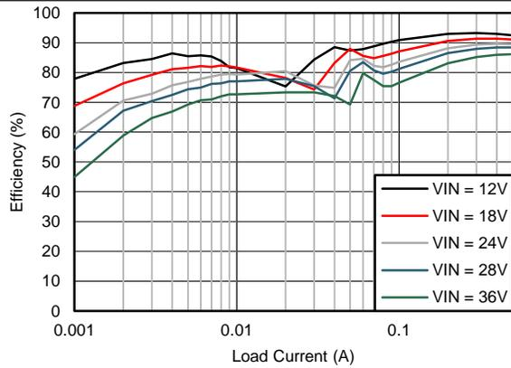
$V_{OUT} = 5\text{ V}$   $F_{SW} = 500\text{ kHz}$
