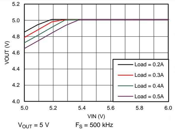
Figure 62. Dropout Curve
