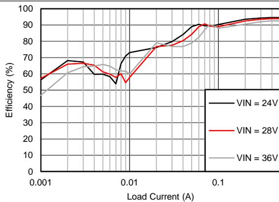
$V_{OUT} = 12\text{ V}$   $F_{SW} = 500\text{ kHz}$
