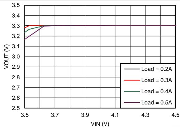
Figure 13. Dropout Curve
