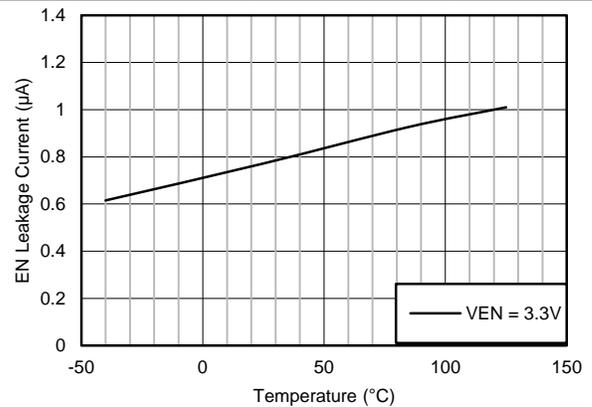
Figure 28. Enable Leakage Current vs Junction Temperature
