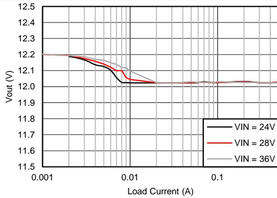
Figure 11.  $V_{OUT}$  Regulation
