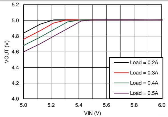
Figure 14. Dropout Curve
