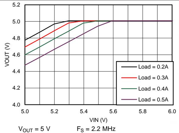
Figure 80. Dropout Curve
