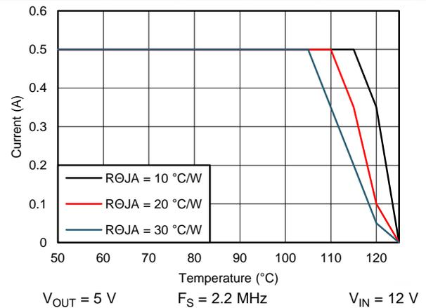
Figure 82. Derating Curve
