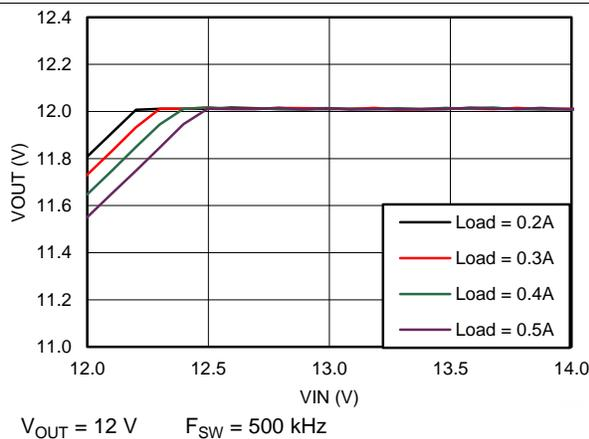
Figure 17. Dropout Curve
