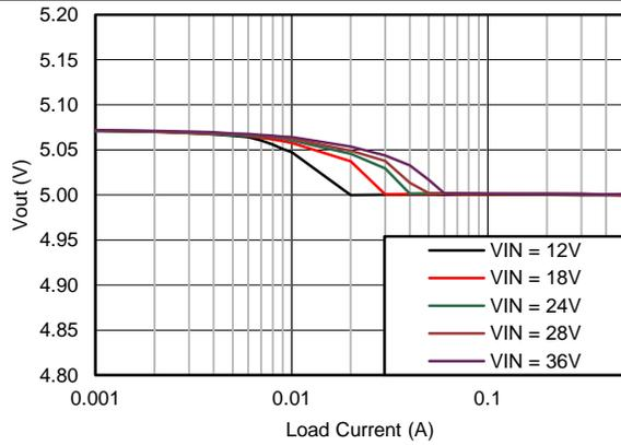
Figure 9.  $V_{OUT}$  Regulation
