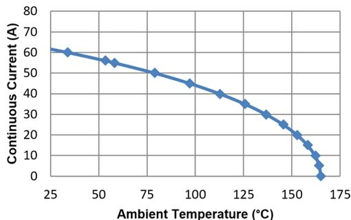
**Figure 5: Maximum Continuous Current at a Given  $T_A$**
