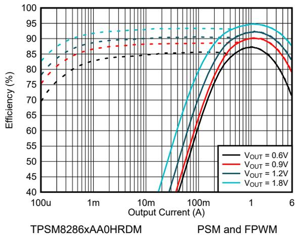
**Figure 9-12. Efficiency  $V_{IN} = 2.8\text{ V}$  and  $T_A = 25^\circ\text{C}$**
