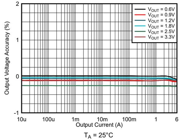
Figure 9-15. Load Regulation  $V_{IN} = 5.0\text{ V}$  and FPWM
