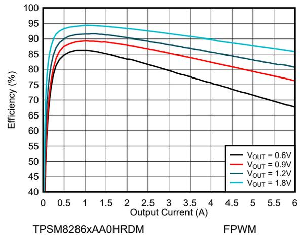
**Figure 9-13. Efficiency  $V_{IN} = 2.8\text{ V}$  and  $T_A = 85^\circ\text{C}$**
