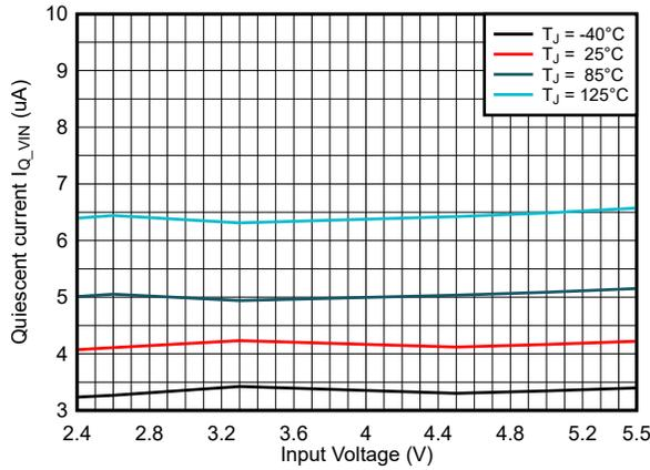
**Figure 7-1. Quiescent Current into V<sub>IN</sub> I<sub>Q\_VIN</sub>**
