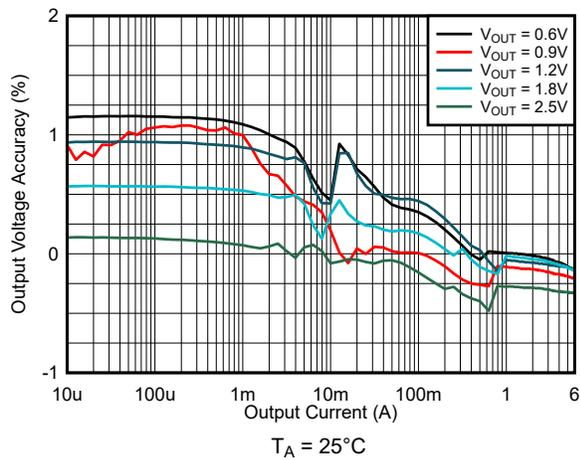
Figure 9-16. Load Regulation  $V_{IN} = 3.3\text{ V}$  and PSM
