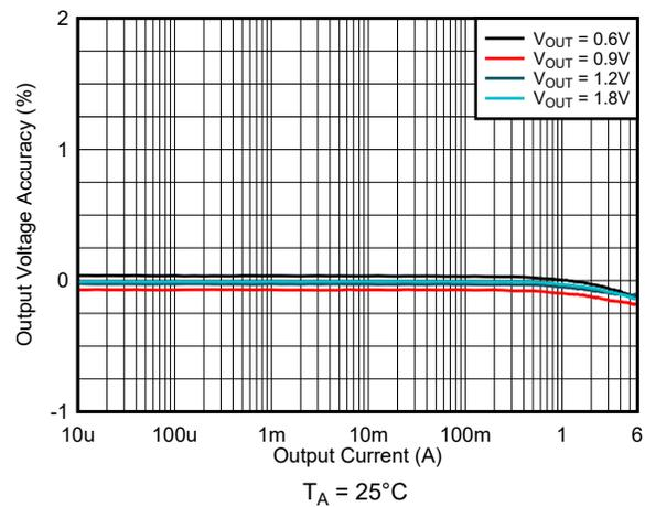
Figure 9-19. Load Regulation  $V_{IN} = 2.8\text{ V}$  and FPWM
