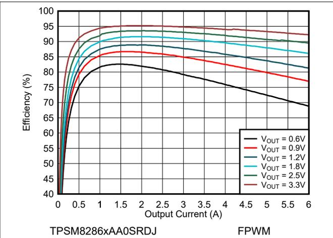
Figure 9-3. Efficiency  $V_{IN} = 5.0\text{ V}$  and  $T_A = 85^\circ\text{C}$
