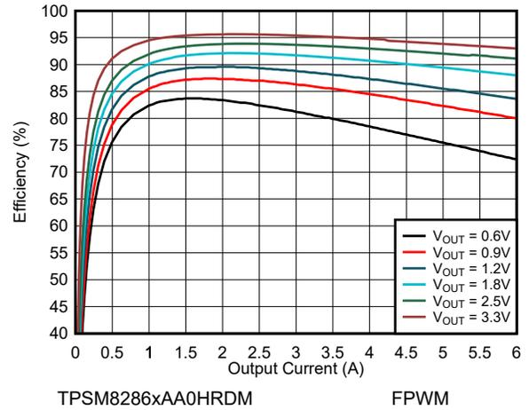
**Figure 9-9. Efficiency  $V_{IN} = 5.0\text{ V}$  and  $T_A = 85^\circ\text{C}$**
