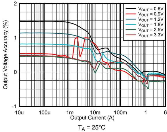
Figure 9-14. Load Regulation  $V_{IN} = 5.0\text{ V}$  and PSM
