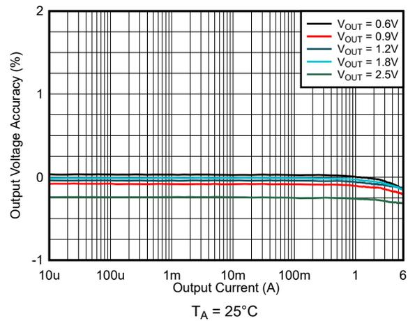
Figure 9-17. Load Regulation  $V_{IN} = 3.3\text{ V}$  and FPWM
