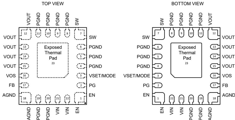
**Figure 6-1. TPSM82864A, TPSM82866A - QFN (23 Pin)**
