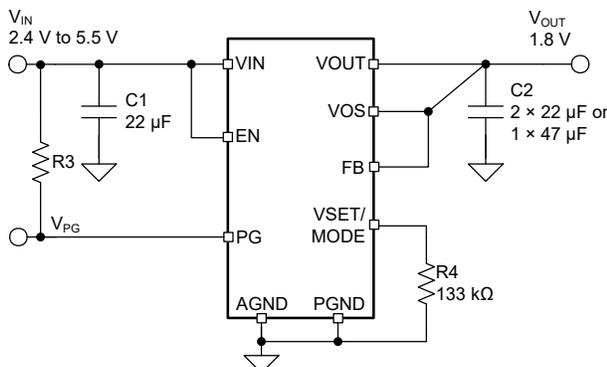
Typical Application Schematic – Fixed Output Voltage Option
