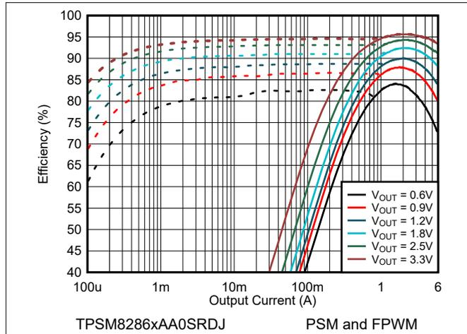
Figure 9-2. Efficiency  $V_{IN} = 5.0\text{ V}$  and  $T_A = 25^\circ\text{C}$
