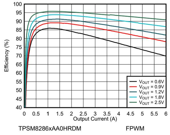
**Figure 9-11. Efficiency  $V_{IN} = 3.3\text{ V}$  and  $T_A = 85^\circ\text{C}$**
