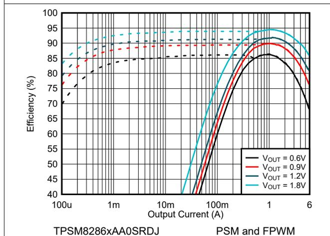
Figure 9-6. Efficiency  $V_{IN} = 2.8\text{ V}$  and  $T_A = 25^\circ\text{C}$
