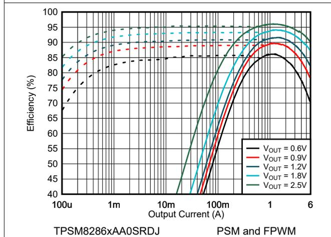
Figure 9-4. Efficiency  $V_{IN} = 3.3\text{ V}$  and  $T_A = 25^\circ\text{C}$
