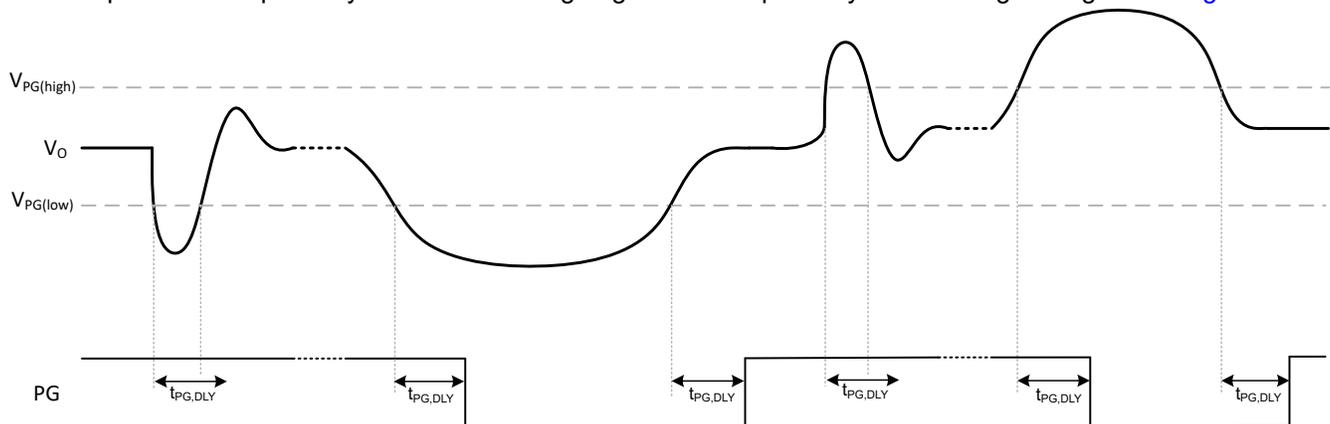
**Figure 8-3. Power-Good Transient and Delay Behavior**
