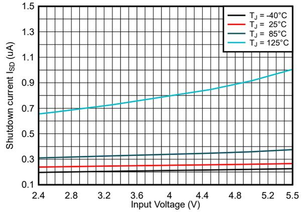
**Figure 7-2. Shutdown Current I<sub>SD</sub>**
