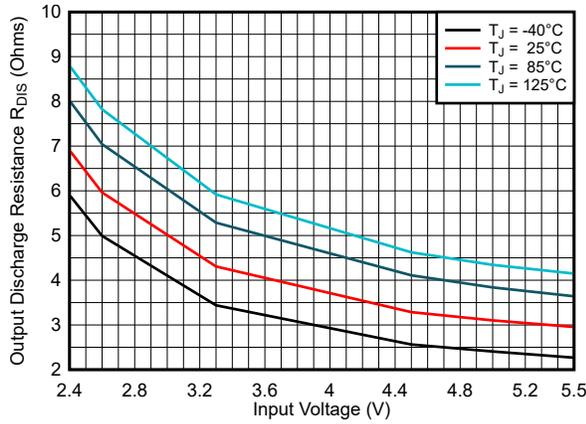
**Figure 7-3. Output Discharge Resistance R<sub>DIS</sub>**
