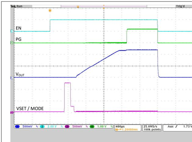
$R_{VSET} = 56.2\text{ k}\Omega$   $I_{OUT} = 6.0\text{ A}$
