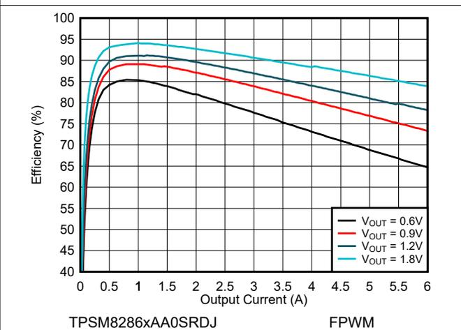
Figure 9-7. Efficiency  $V_{IN} = 2.8\text{ V}$  and  $T_A = 85^\circ\text{C}$
