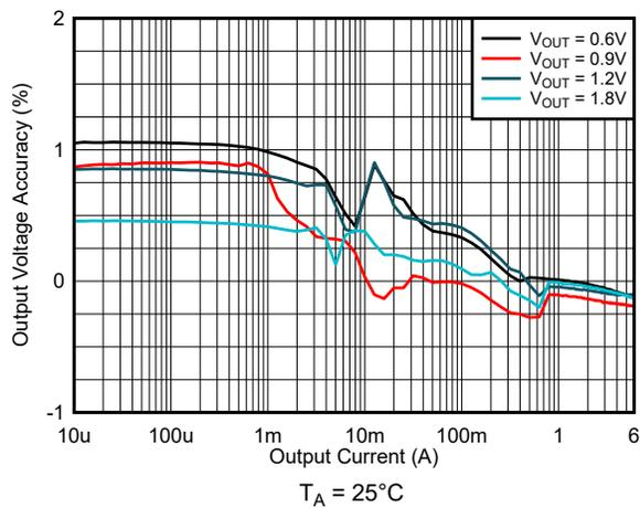
Figure 9-18. Load Regulation  $V_{IN} = 2.8\text{ V}$  and PSM
