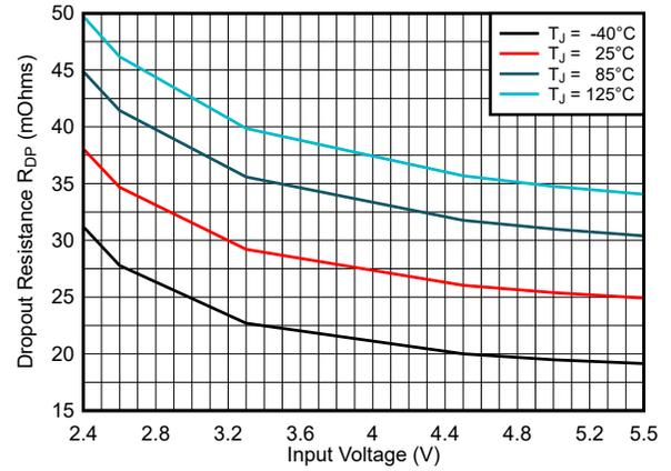
**Figure 7-4. Dropout Resistance R<sub>DP</sub>**
