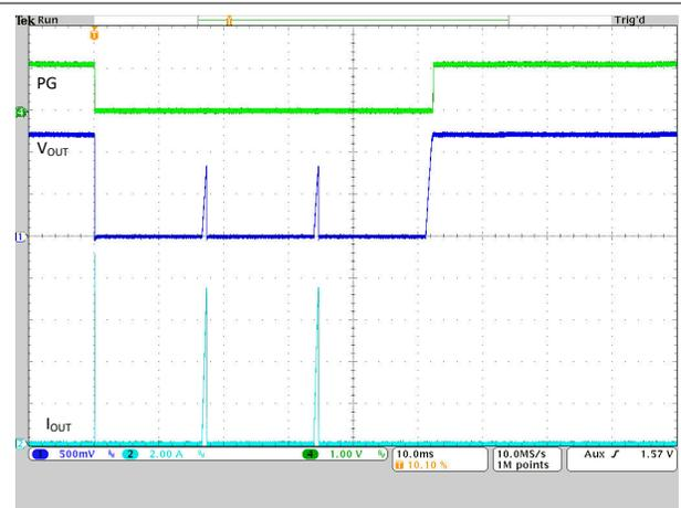
$R_{LOAD} = 100\text{ m}\Omega$  (during overload)
