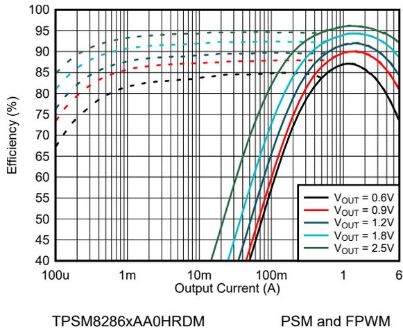
**Figure 9-10. Efficiency  $V_{IN} = 3.3\text{ V}$  and  $T_A = 25^\circ\text{C}$**
