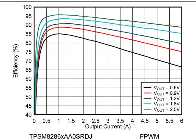
Figure 9-5. Efficiency  $V_{IN} = 3.3\text{ V}$  and  $T_A = 85^\circ\text{C}$
