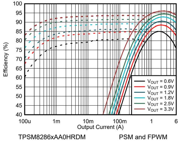
**Figure 9-8. Efficiency  $V_{IN} = 5.0\text{ V}$  and  $T_A = 25^\circ\text{C}$**
