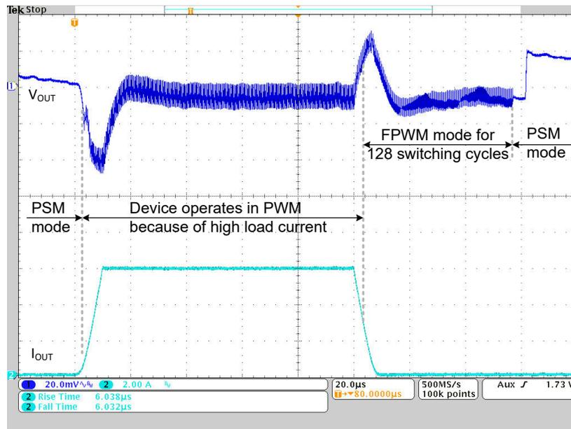
Figure 8-1. Optimized Transient Performance from PWM to PSM
