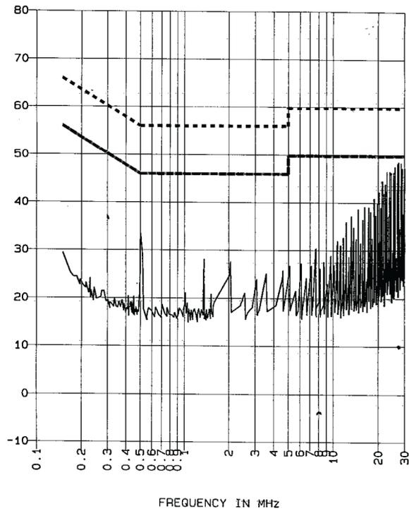
Figure 9. JW075A1 Conducted Noise with Filter 8-1387(F)
