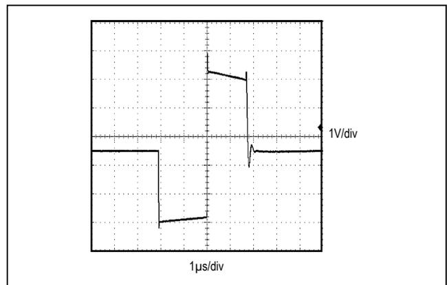
Figure 6. LX Ringing With Damping Switch (MAX1722/MAX1724)
