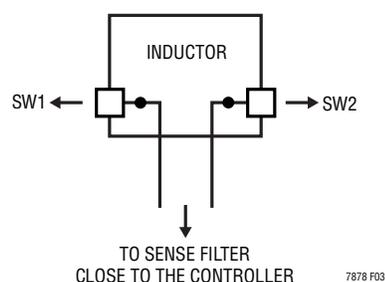
Figure 3. Sense Lines Placement with Inductor DCR
