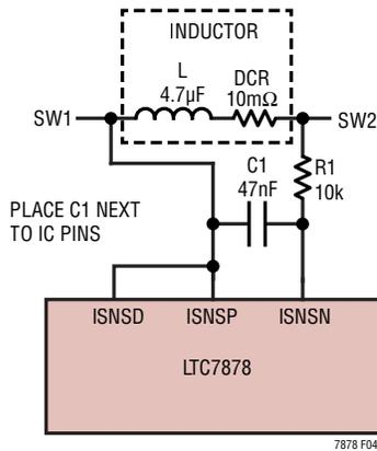
Figure 4. Inductor DCR Current Sensing
