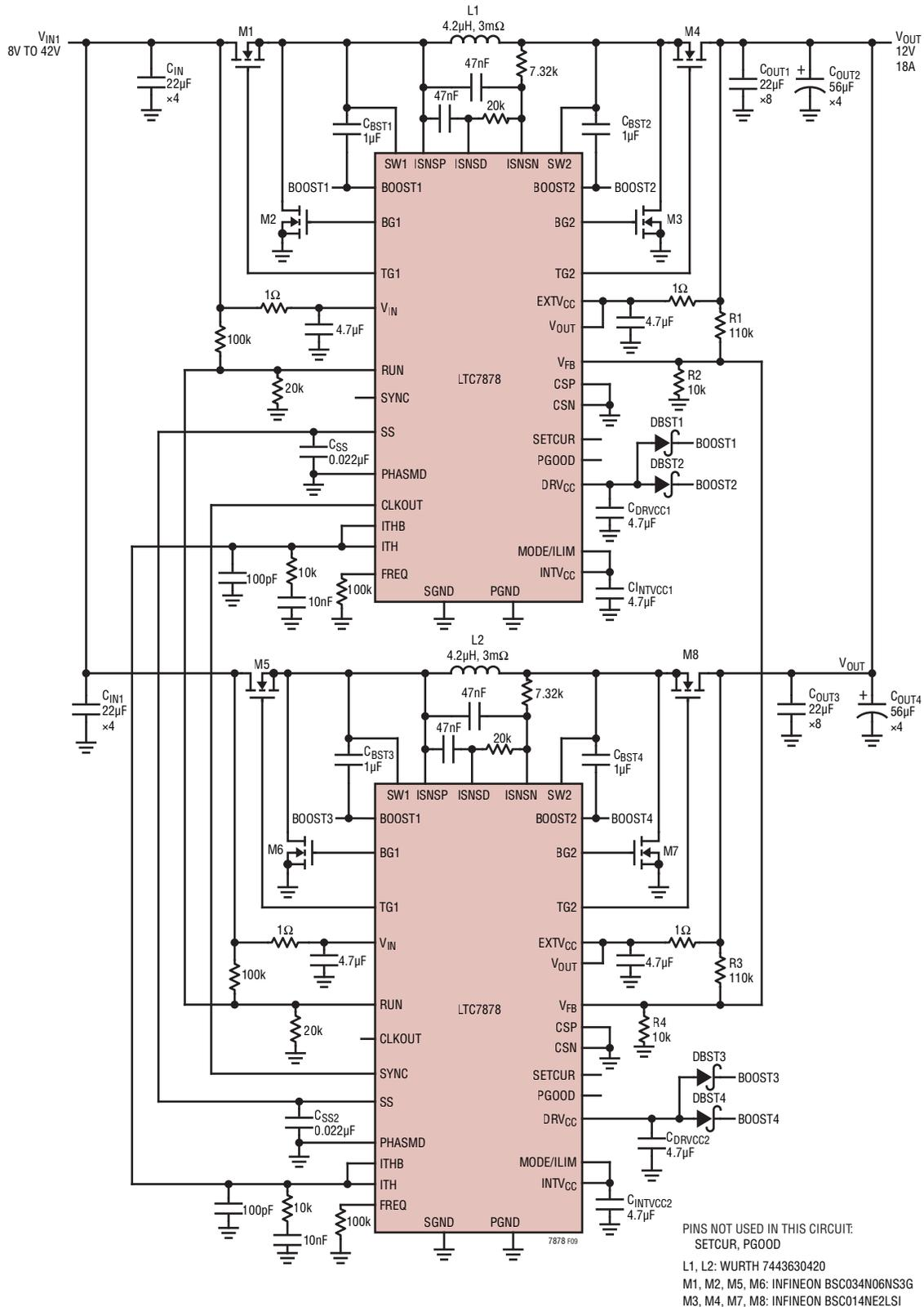
Figure 9. Two-Phase Parallel Operation 12V<sub>OUT</sub>/18A Buck-Boost Converter
