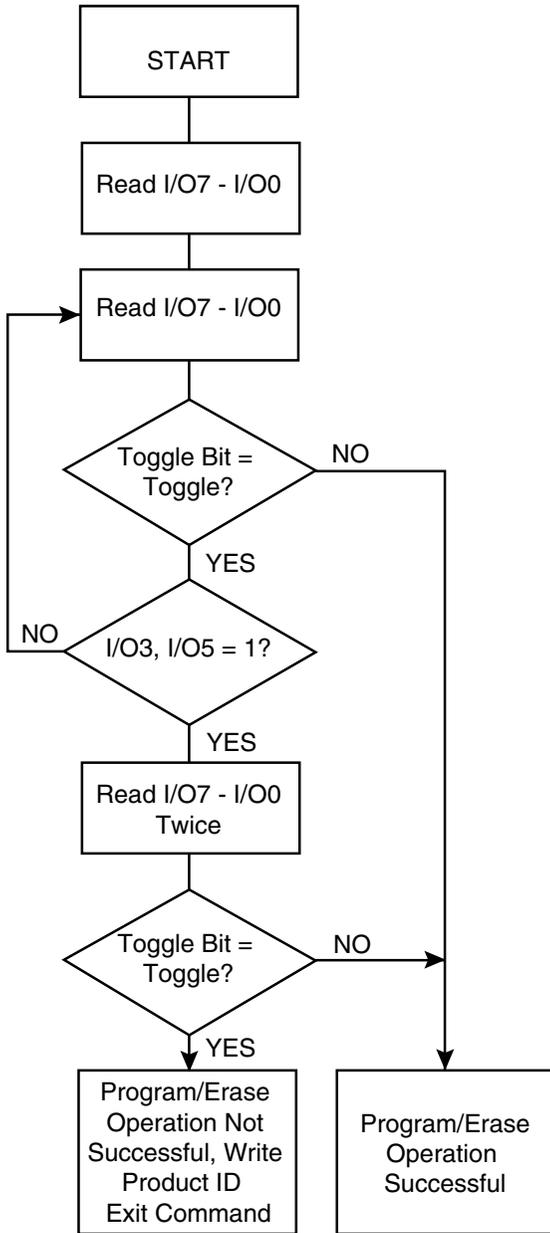
**Figure 4.** Toggle Bit Algorithm
