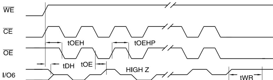
Notes: 1. Toggling either  $\bar{O}\bar{E}$  or  $\bar{C}\bar{E}$  or both  $\bar{O}\bar{E}$  and  $\bar{C}\bar{E}$  will operate toggle bit. The  $t_{OEHP}$  specification must be met by the toggling input(s).
