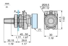
e: clamping thickness: 1 mm to 6 mm / 0.03 in. to 0.24 in.
