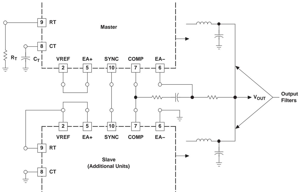
NOTE: Slaving allows parallel operation of two or more units with equal current sharing.
