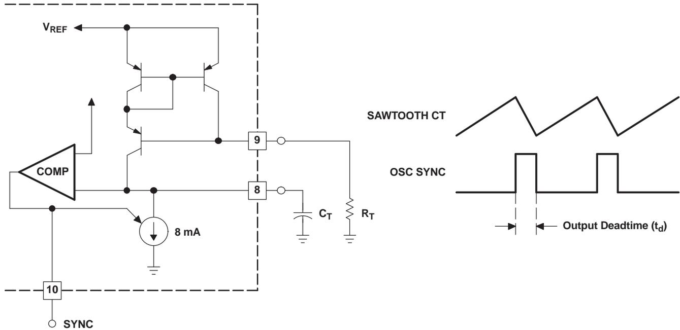
NOTE: Output deadtime is determined by the size of the external capacitor,  $C_T$ , according to the formula:  $T_d = \frac{2C_T}{8 \text{ mA} - \frac{3.6}{R_T}}$
