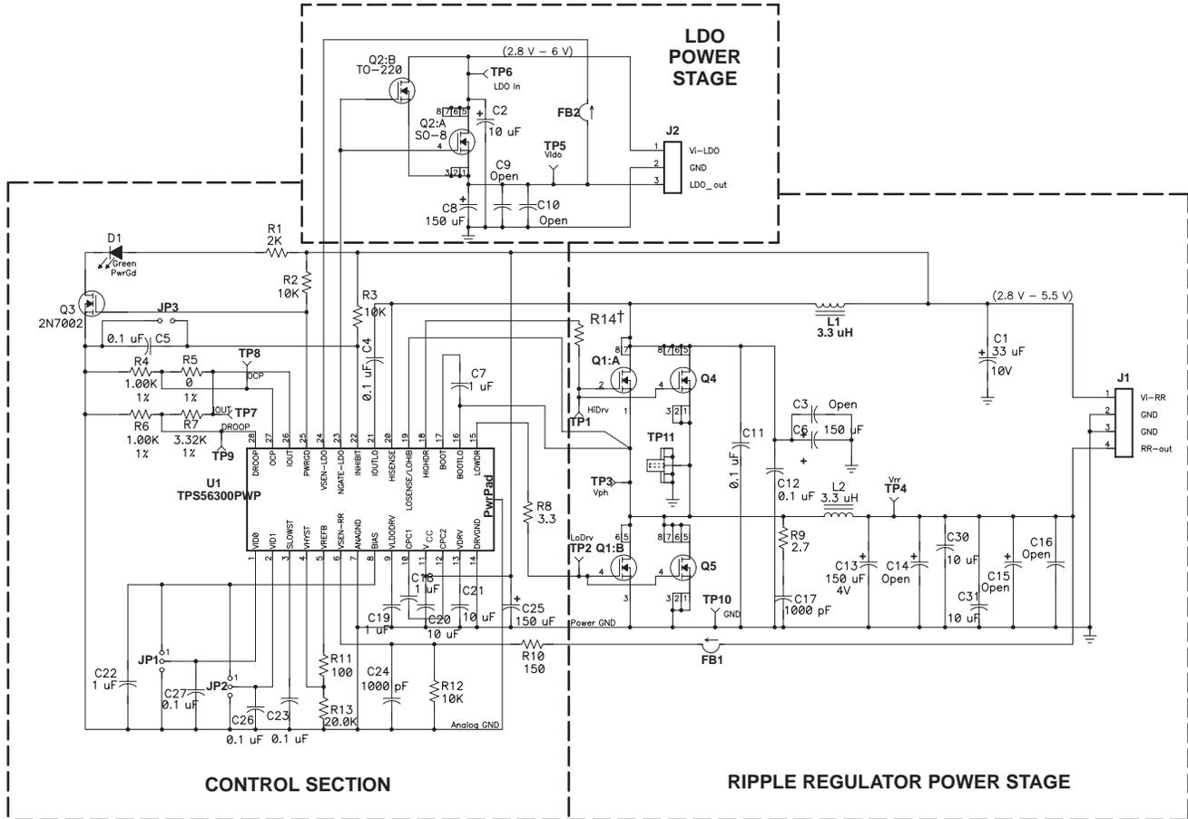
† When an output current greater than 4 A is desired on the ripple regulator, please add a 10 Ω resistor (R14) between pin 18 and Q1:A. Because the EVM is configured for 4 A and below, R14 is 0 Ω and is not included on the module.
