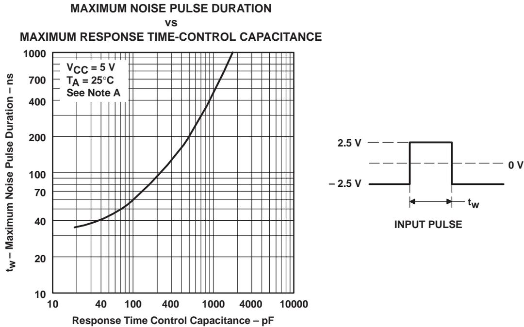
NOTE A: Figure 11 shows the maximum duration of the illustrated pulse that can be applied differently without the output changing from the low to high level.
