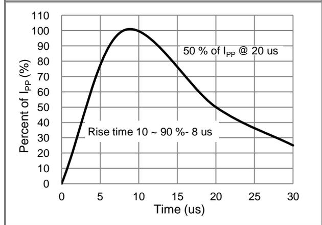
Fig.2 Pulse Waveform
