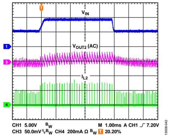
Figure 42. Channel 2 Line Transient in Hysteresis Mode
