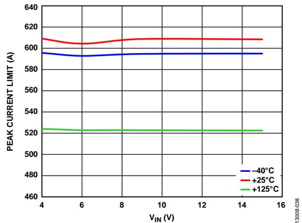
Figure 38. Channel 2 Peak Current Limit vs.  $V_{IN}$
