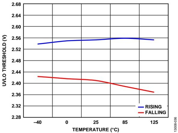
Figure 36. UVLO Threshold, Rising and Falling, vs. Temperature
