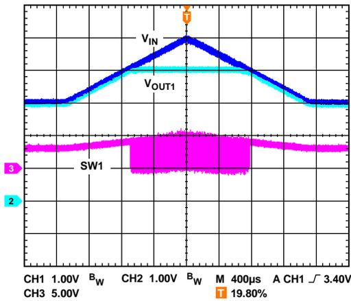
Figure 48. Channel 1 100% Duty Operation in PWM Mode
