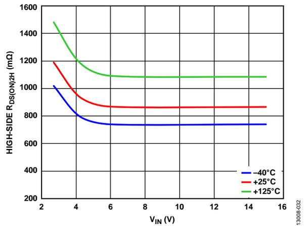
Figure 32. Channel 2 High-Side  $R_{DS(ON)2H}$  vs.  $V_{IN}$
