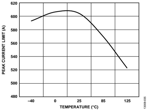
Figure 35. Channel 2 Peak Current Limit vs. Temperature
