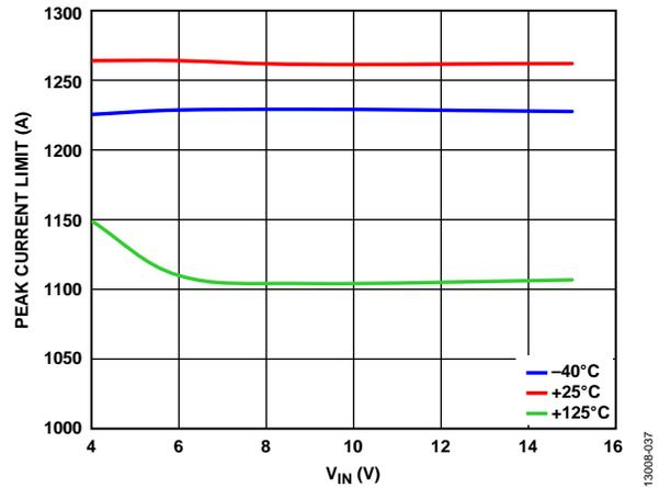
Figure 37. Channel 1 Peak Current Limit vs.  $V_{IN}$
