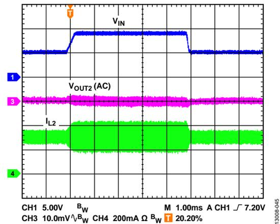
Figure 45. Channel 2 Line Transient in PWM Mode
