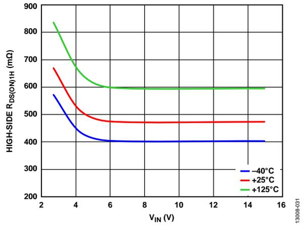
Figure 31. Channel 1 High-Side  $R_{DS(ON)1H}$  vs.  $V_{IN}$
