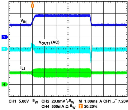
Figure 46. Channel 1 Line Transient in PWM Mode
