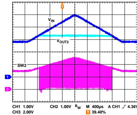
Figure 51. Channel 2 100% Duty Operation in PWM Mode
