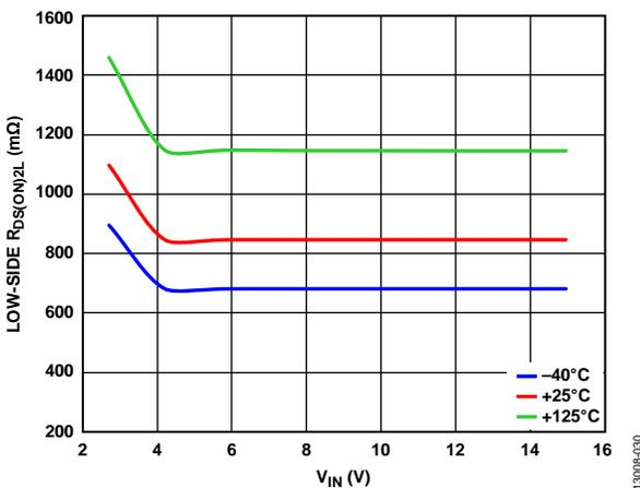
Figure 30. Channel 2 Low-Side  $R_{DS(ON)2L}$  vs.  $V_{IN}$
