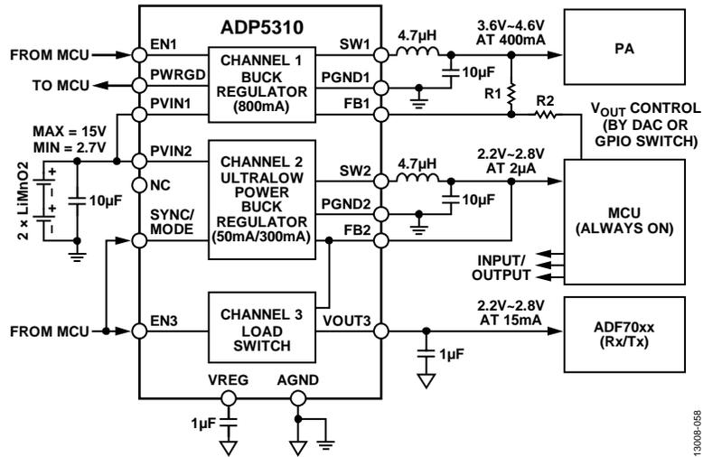
Figure 58. Typical Application of a Smart Meter
