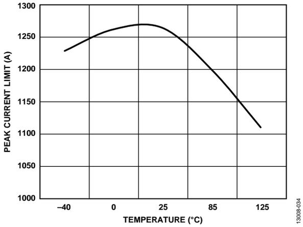
Figure 34. Channel 1 Peak Current Limit vs. Temperature
