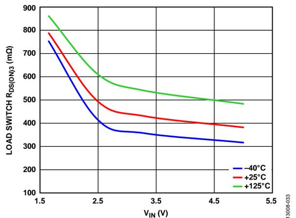
Figure 33. Channel 3 Load Switch  $R_{DS(ON)3}$  vs.  $V_{IN}$
