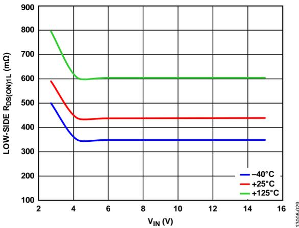
Figure 29. Channel 1 Low-Side  $R_{DS(ON)1L}$  vs.  $V_{IN}$
