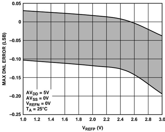
Figure 8. DNL vs.  $V_{REFP}$  ( $V_{SUPPLY} = +5 V$ )
