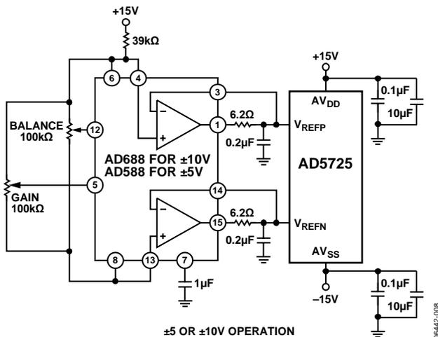
Figure 28. Symmetrical Bipolar Operation
