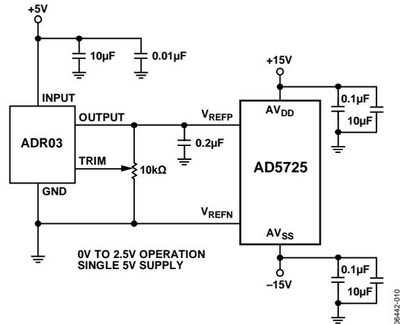
Figure 30.  $+5\text{ V}$  Single-Supply Operation
