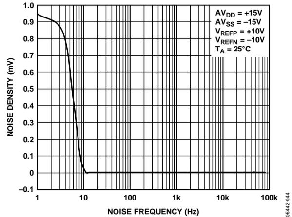
Figure 22. Output Noise Spectral Density vs. Frequency
