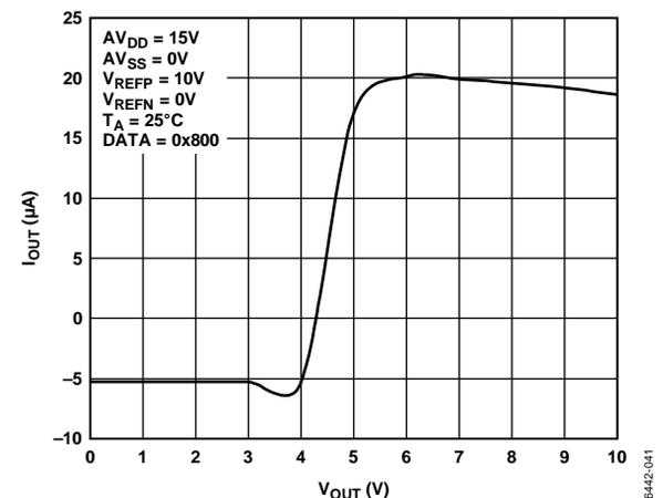
Figure 24.  $I_{OUT}$  vs.  $V_{OUT}$  ( $V_{SUPPLY} = +15 V$ )
