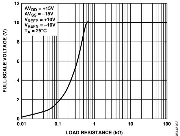
Figure 19. Output Voltage Swing vs. Resistive Load
