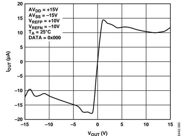
Figure 23.  $I_{OUT}$  vs.  $V_{OUT}$  ( $V_{SUPPLY} = \pm 15 V$ )
