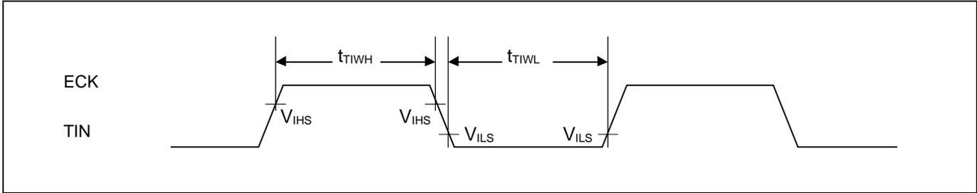
■ Trigger input timing
