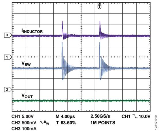
Figure 18. Skip Mode Operation Showing Inductor Current ( $I_{INDUCTOR}$ ), Switch Node Voltage ( $V_{SW}$ ), and Output Ripple ( $V_{OUT}$ ),  $V_{IN} = 12\text{ V}$ ,  $V_{OUT} = -5\text{ V}$ ,  $I_{LOAD} = 1\text{ mA}$ ,  $f_{SW} = 1.2\text{ MHz}$ ,  $T_A = 25^\circ\text{C}$
