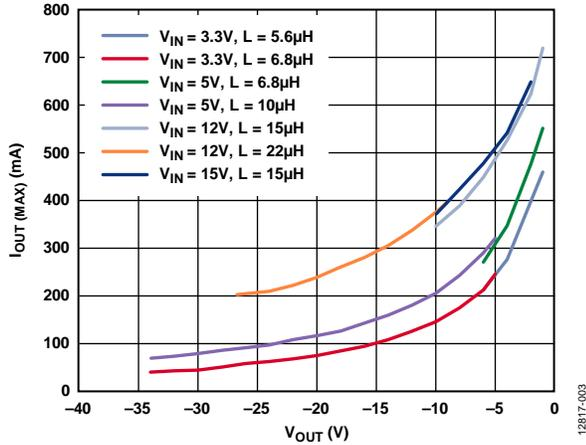
Figure 3. Maximum Output Current,  $f_{SW} = 1.2$  MHz,  $T_A = 25^\circ C$ , Based on Target of 70%  $I_{LIM(MIN)}$
