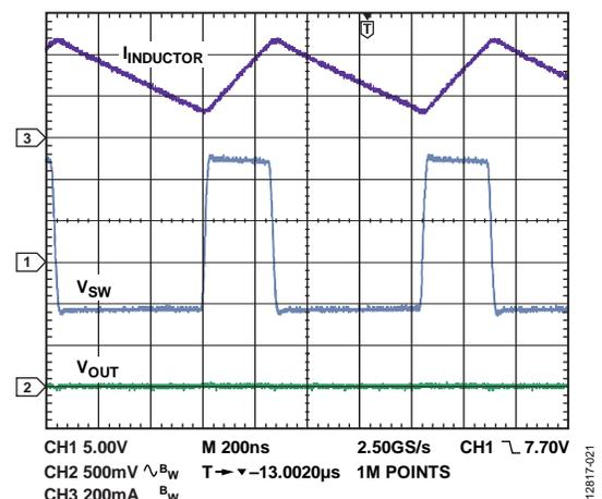
Figure 20. Continuous Conduction Mode Operation Showing Inductor Current ( $I_{INDUCTOR}$ ), Switch Node Voltage ( $V_{SW}$ ), and Output Ripple ( $V_{OUT}$ ),  $V_{IN} = 12\text{ V}$ ,  $V_{OUT} = -5\text{ V}$ ,  $I_{LOAD} = 200\text{ mA}$ ,  $f_{SW} = 1.2\text{ MHz}$ ,  $T_A = 25^\circ\text{C}$
