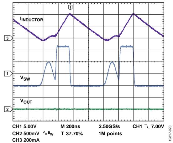
Figure 19. Discontinuous Conduction Mode Operation Showing Inductor Current ( $I_{INDUCTOR}$ ), Switch Node Voltage ( $V_{SW}$ ), and Output Ripple ( $V_{OUT}$ ),  $V_{IN} = 12\text{ V}$ ,  $V_{OUT} = -5\text{ V}$ ,  $I_{LOAD} = 50\text{ mA}$ ,  $f_{SW} = 1.2\text{ MHz}$ ,  $T_A = 25^\circ\text{C}$
