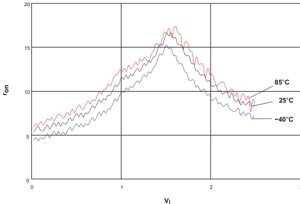
**Figure 12.**  $r_{on}$  vs  $V_I$ ,  $V_{CC} = 2.5$  V (SN74LVC1G66-Q1)
