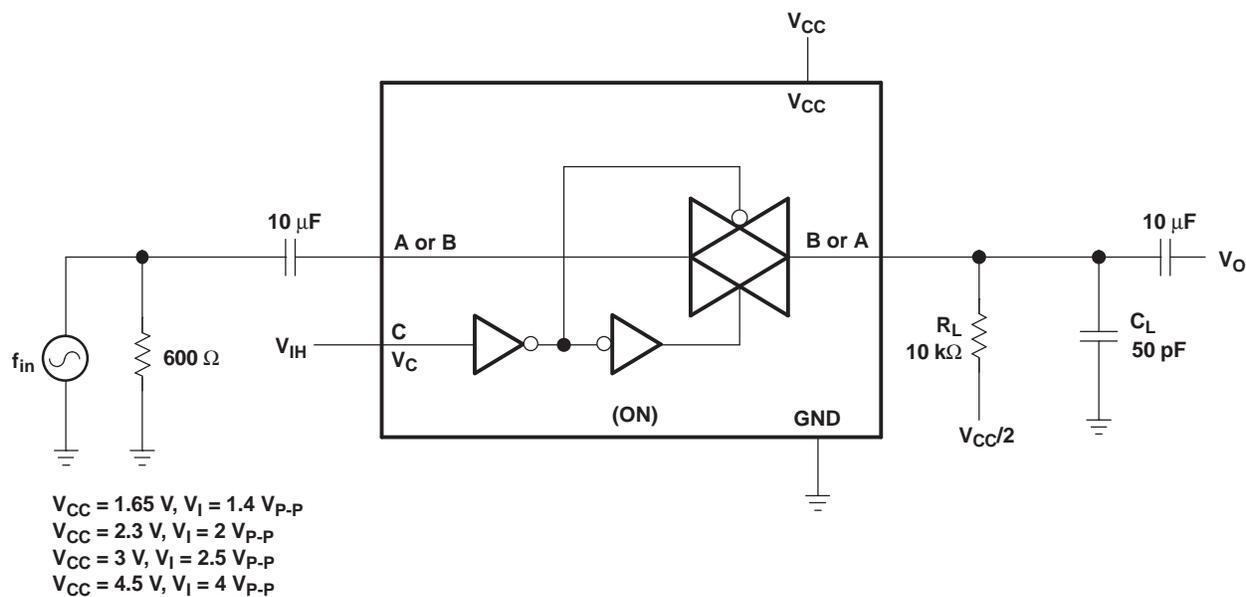
Figure 9. Sine-Wave Distortion
