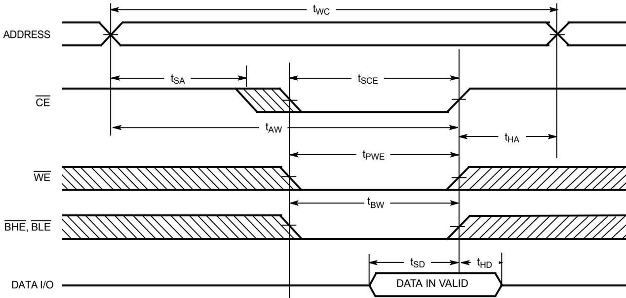
Figure 7. Write Cycle 2 ( $\overline{\text{WE}}$  Controlled,  $\overline{\text{OE}}$  LOW) [16, 17]
