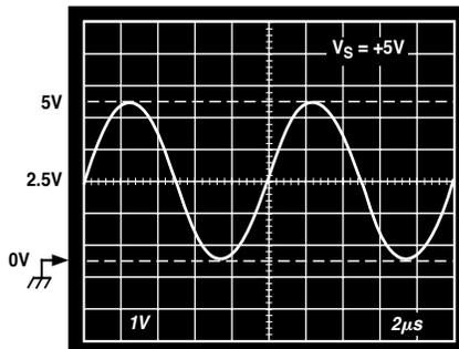
Figure 1. Output Swing: Gain =  $-1$ ,  $R_L = 2 \text{ k}\Omega$
