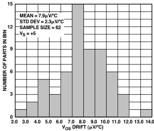
Figure 5.  $V_{OS}$  Drift Over  $-40^{\circ}\text{C}$  to  $+85^{\circ}\text{C}$
