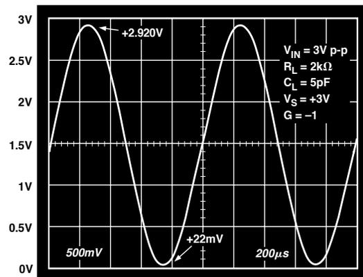
Figure 31. Output Swing,  $V_S = +3\text{ V}$
