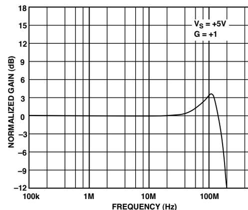
Figure 2. Frequency Response: Gain =  $+1$ ,  $V_S = +5 \text{ V}$
