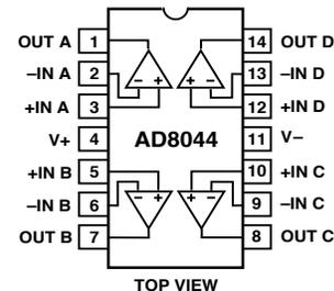
The output voltage swing extends to within 25 mV of each rail, providing the maximum output dynamic range. Additionally, it features gain flatness of 0.1 dB to 12 MHz, while offering differential gain and phase error of 0.04% and 0.22° on a single +5 V supply. This makes the AD8044 useful for video electronics, such as cameras, video switchers, or any high speed portable equipment. The AD8044's low distortion and fast settling make it ideal for active filter applications.
